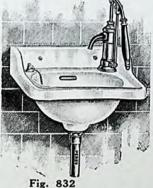
With integral back and round basin. Complete with chromium plated waste plug, chainstay, chain, and stopper. Size of outlet 11/4 inch outside diameter.
