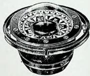
The spherical dome magnifies the card and provide unusual stability. Non-glare and non-shadow und lighting.
