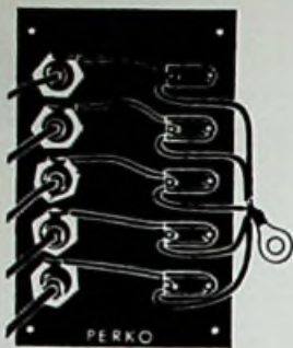
BACK VIEW OF IMPROVED PANEL
