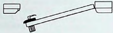
Left Hand Door Showing Reverse Bevel Lock With Non-Interchangeable Knob and Lever.
