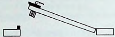
Left Hand Door Showing Regular Bevel Lock With Non-Interchangeable Knob and Lever.
