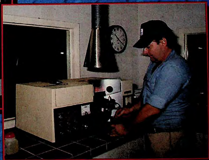
Below: Quality Control Lab Utilizing Atomic Absorption Spectrophotometry
