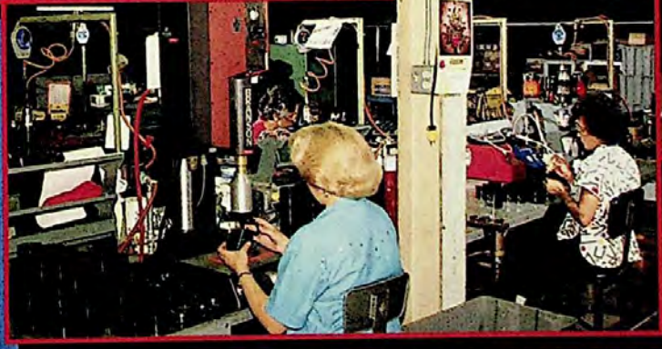
Left: Ultrasonic Bonding of Navigation Light Lenses
