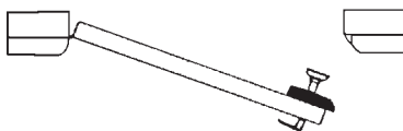
Right Hand Door Showing Reverse Bevel Lock With Interchangeable Knob and Lever.
