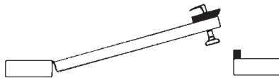
Right Hand Door Showing Regular Bevel Lock With Interchangeable Knob and Lever.
